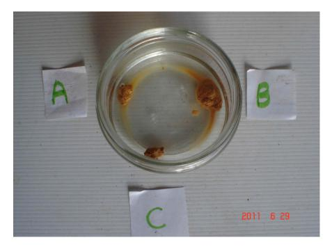
The next graphic shows the samples at 2 hours, sample A has begun to collapse, sample B has completely dispersed but sample C had only slight slaking.
